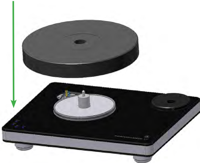
Pic. 8: Setting the platter onto the bearing
